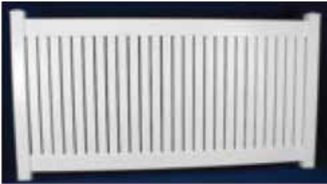
3" Semi-Privacy Rails: 1-1/2" x 5-1/2" top and bottom rail (reinforced) 2" x 3-1/2" mid rail (on 6' height only) Pickets: 7/8" x 3" pickets Picket space = 1/2"
